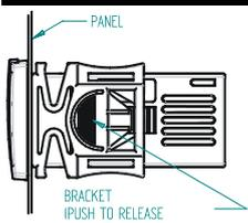
Instrument **XR40CX** shall be mounted on vertical panel, in a 29x71 mm hole, and fixed using the special bracket supplied. The temperature range allowed for correct operation is 0+60 °C. Avoid places subject to strong vibrations, corrosive gases, excessive dirt or humidity. The same recommendations apply to probes. Let air circulate by the cooling holes.
