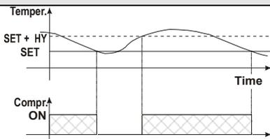
In case of fault in the thermostat probe the start and stop of the compressor are timed through parameters "COOn" and "COF".
