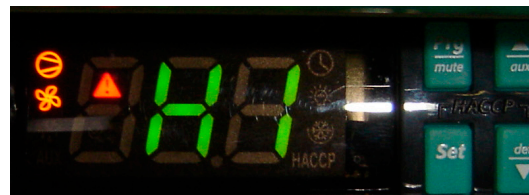
This image shows the controller during an alarm condition. This is the high temperature alarm code (HI). Other codes may also be displayed. (See above for other codes)
