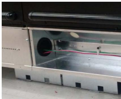
**FIGURE 52: Electrical Supply Access Hole**
