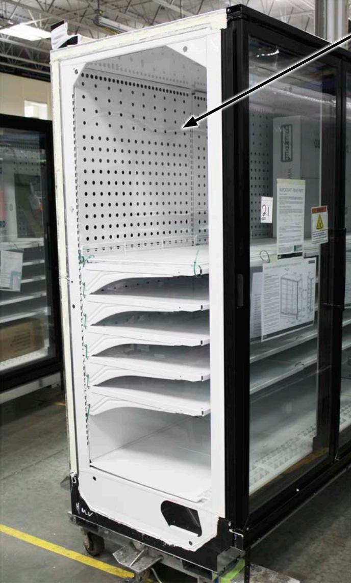
Clear plexi dividers separate refrigeration circuits between same temperature cases.
