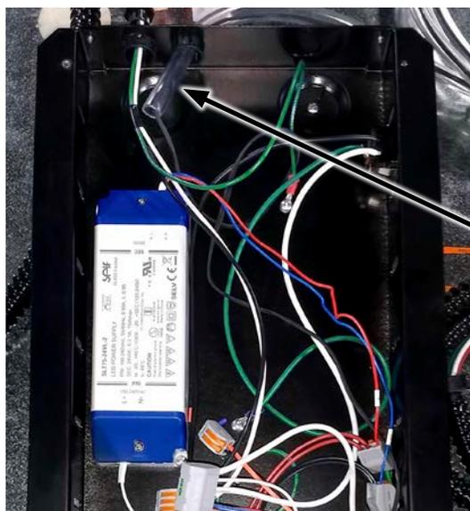
Connect sensor wires
