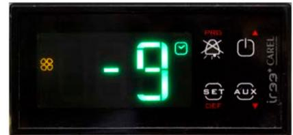
1. Press and hold the [PRG] button down for 5 seconds. The display will show a flashing "0". Once "0" is flashing, press [UP] arrow until you see "22". Press [SET] button to enter this access number to get to these parameters.
