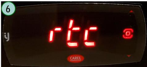
6. Navigate using the [UP] and [DOWN] arrows to select "Rtc" for the real time clock (See #6). Touch the [PRG] button.
