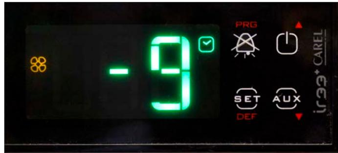
The Carel IR33+ controller has a two-level menu system for programming the operation of the case; Level 1 and Level 2 program settings.
