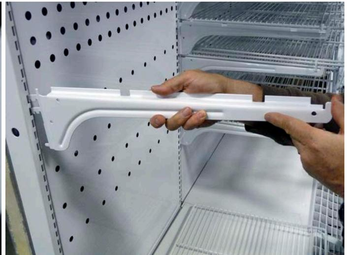
**REMOVAL:** Lift the front of the shelf, then lift the back of the shelf. Tilt the front of the shelf bracket up and pull the shelf bracket tabs clear of the shelf standard. Repeat the process for the opposite shelf bracket.
