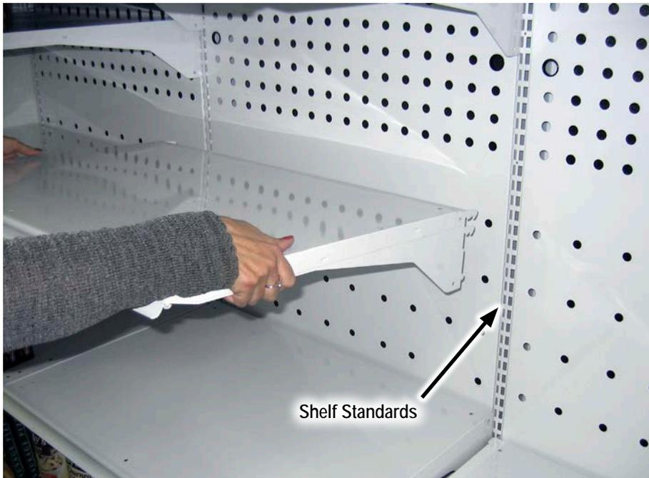
**INSTALLATION:** Determine desired shelving location. Lift the front of the shelf at a slight angle, keeping the shelf level left to right. Insert the shelf tabs into the slots in the shelf standards. Lower the front of the shelf while moving the shelf tabs into the standards and until the shelf is held securely by the standards.
