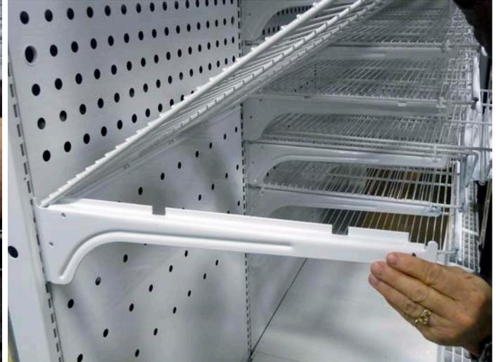
**INSTALLATION:** Determine desired bracket and shelving location. With the first bracket, lift the front of it up at a slight angle. Insert the shelf bracket tabs into the slots in the shelf standard. Lower the front of the shelf bracket while moving the tabs into the standards and until the shelf bracket is held securely by the standard.
