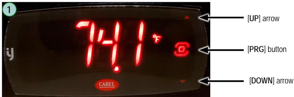
2. Touch and hold the [PRG] button down until the display shows three dashes " - - - " that stay steady (See #2).
