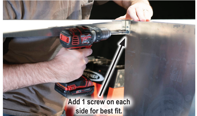
FIGURE 8: Mount the Signage Rail to the Divider
