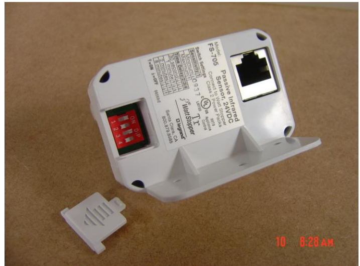
Picture 2. The back of the sensor showing the dip switches.
