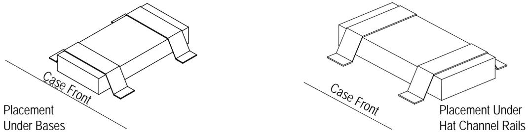
FIGURE 9: Shims Under Bases (Without Hat Channel Rails)
