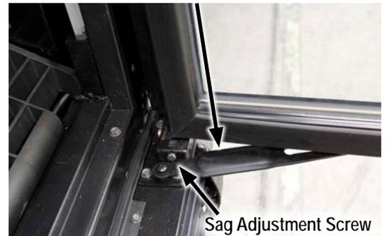
The hold-open bracket is located on the bottom of the door on Crystal™ freezers (See Figure 24).
