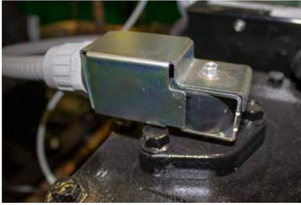
FIGURE 25: Mechanical Unloader
