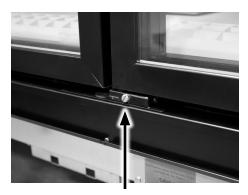
**FIGURE 4: Door Tension Screw**
