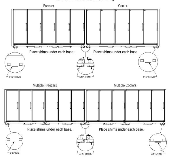
FIGURE 14: Cooler to Freezer Leveling
