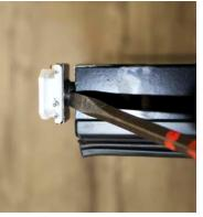
FIGURE 30: Remove Torque Rod
