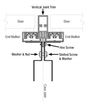
Apply caulk between joints. Attach vertical joint trim using the hex screws. Join cases using joint hardware.
