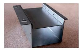
Spacer blocks are factory-installed in the end bases of 4 or 5-door cases that use bases taller than 3 1/2". These blocks limit the case's forward tilt while it is being lifted by a forklift (See Figure 4).
