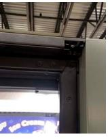
FIGURE 32: Hinge Pin Bracket
