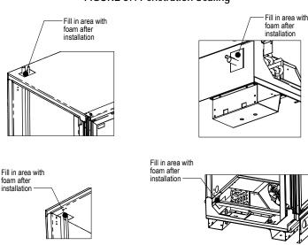
FIGURE 37: Penetration Sealing
