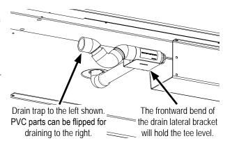
FIGURE 20: Drain Installation
