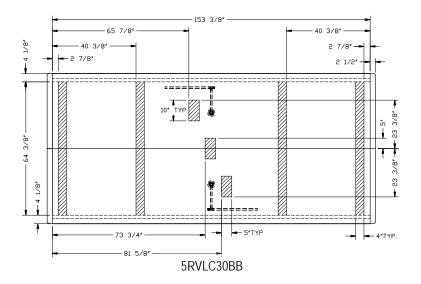
7. To maintain even, consistent gaps and proper door operation, the case must be leveled front-to-back and side-to-side. Ensure that the case is set square to within 1/8" (See Figure 12). After the case is set, use at least a 48" level to ensure the case is level. Add additional shims as needed under specific bases.
