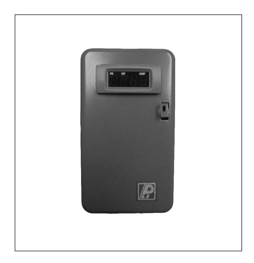
The **ERC 2 Electronic Refrigeration Control** is a microprocessor-based electronic controller designed to control both the temperature and the defrost functions of a commercial refrigeration unit. It can be powered by 120, 208 or 240 VAC (50 or 60Hz). The control comes with four relay outputs: compressor, defrost, evaporator fan and alarm.
