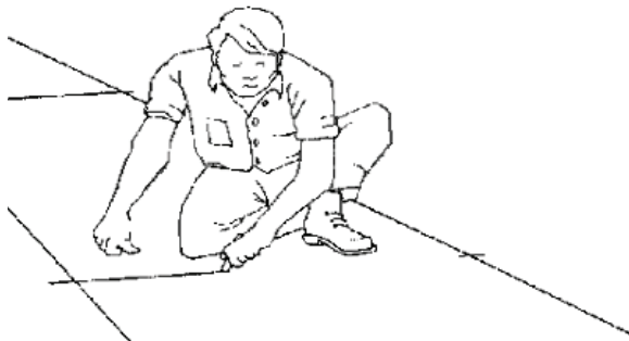
FIGURE 4: Measure and Mark Exact Case Outline
