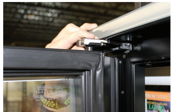
FIGURE 26: Push Door & Hinge Pin into Place
