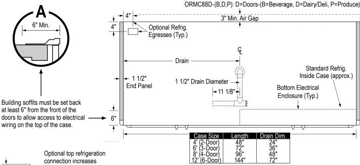
Optional top refrigeration connection increases - case height by up to 4". 68 3/8" Interior Height 74" Door 88 1/2" Case Height 24" 30" ≅ ₹ 4 1/2" Base 3 1/8" Drain 33 5/8" Drain 35 1/4" Kickplate 44 3/8" Handle
