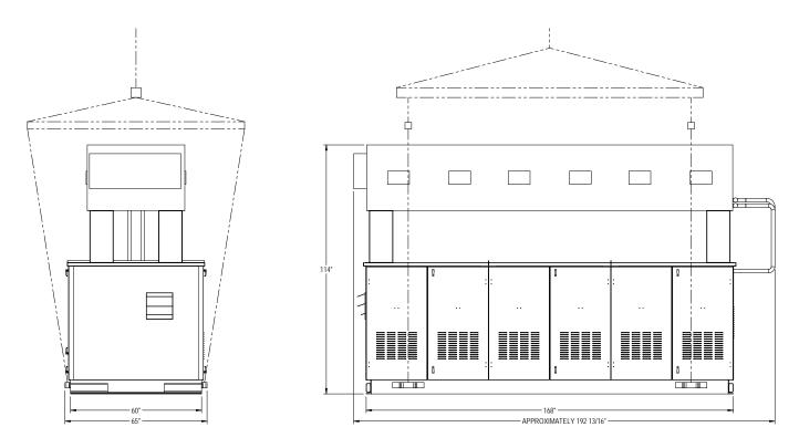
Lift the system using spreader bars to prevent damage to the unit, electrical panels, and piping. All lifting points must be used to distribute the weight evenly to prevent the system from sagging during lifting. When lifting with a crane or hoist, lift slowly to ensure the system is balanced. Systems can be top or front heavy, especially if compressors are double stacked.
