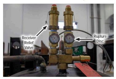
FIGURE 50: Receiver Relief Valve and Rupture Disc
