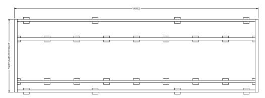
FIGURE 3: Sample Recommended Isolation Pad Locations
