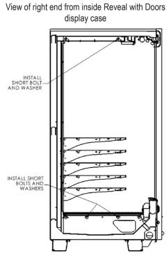
FIGURE 15: Through Bolt Locations Exploded view of right end of Reveal display case
