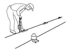
Place enough shims under each base to equal the highest point. Shims should not extend beyond the front case bases or they will interfere with installing trim. The shims should be oriented to sit under the front and rear bends of each base. Tape all shims in place (See Figure 7). After the case is set, additional shims may need to be added at specific base locations (See Figure 9 on page 7).
