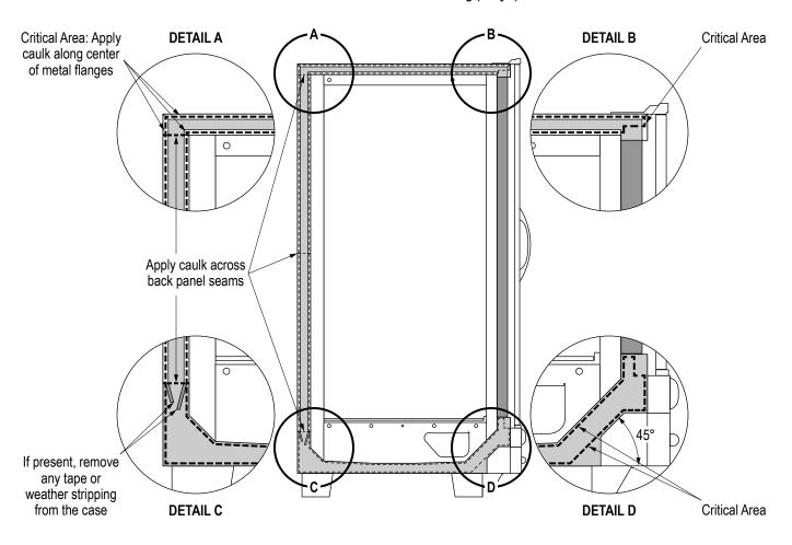
FIGURE 11: Case Joint Caulking (Butyl\*)
