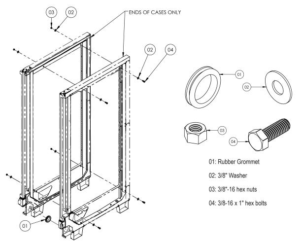
Before joining the cases, remove all packaging material on the display case, including any spacer blocks inside the bases. Repeat caulking between each case in the lineup.
