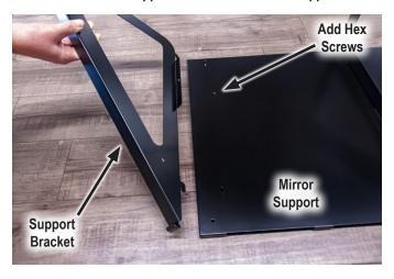
FIGURE 27: Install Mirror Support into the Shelf Standards
