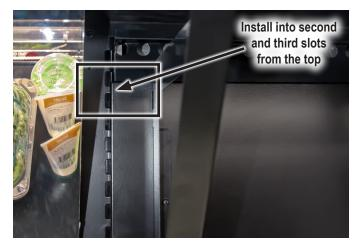
FIGURE 28: Shelf Standard Slots for Air Deflector
