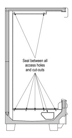
FIGURE 13: NSF Compliance Sealing (Silicone)
