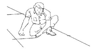
FIGURE 6: Mark Floor Level Difference
