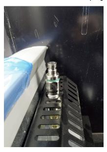
FIGURE 34: Spray Hose Connected
