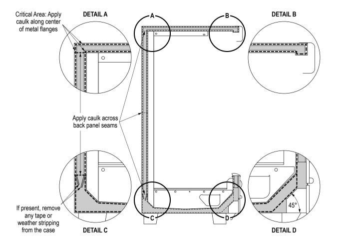
FIGURE 12: Case Joint Caulking (Butyl\*)
