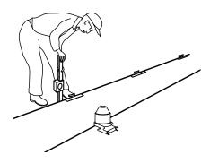
5. Place enough shims under each base to equal the highest point. Shims should not extend beyond the front case bases or they will interfere with installing trim. The shims should be oriented to sit under the front and rear bends of each base. Tape all shims in place (See Figure 7). After the case is set, additional shims may need to be added at specific base locations (See Figure 9 on page 7).
