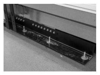
FIGURE 1: Holes Drilled for Rear Bracket
