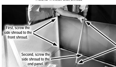
FIGURE 4: Install Side Shroud
