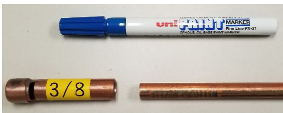
FIGURE 24: Pipe Marking Tool and Paint Marker
