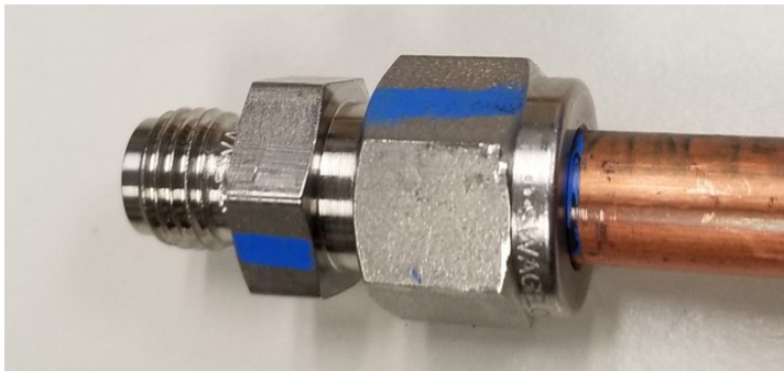
FIGURE 28: Swagelok Properly Tightened
