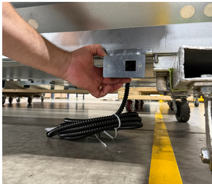
FIGURE 8: Fit Bracket onto Case Edge
